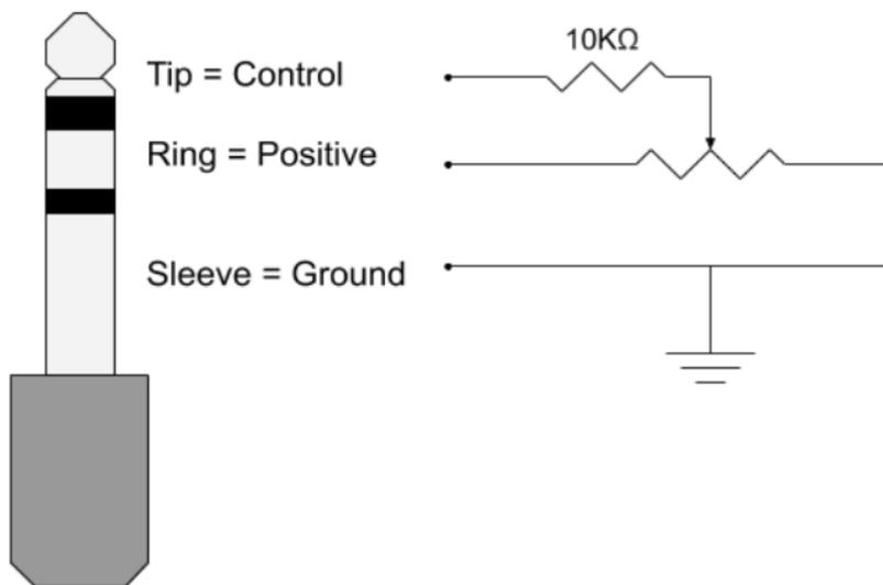
The following diagram shows how to create a cable to convert a volume pedal to an expression pedal.
